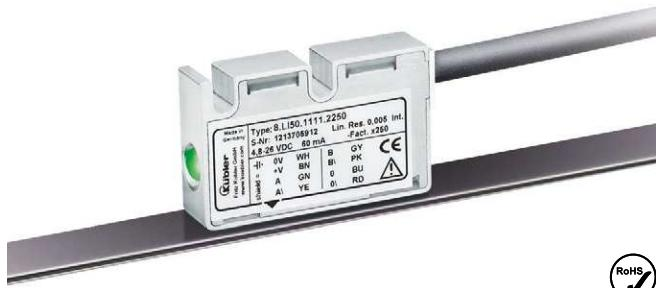
The non-contact incremental magnetic linear measurement system Limes LI50 / B2 - made up of the sensor head LI50 and of the magnetic band B2 - reaches a resolution up to 5 µm with a maximum distance of 2 mm between the sensor and the band.
