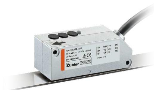
The non-contact absolute magnetic linear measurement system Limes LA50 / BA5 - made up of the sensor head LA50 and of the magnetic band BA5 - reaches a resolution up to 10 µm with a maximum distance of 1.5 mm between the sensor and the band.
