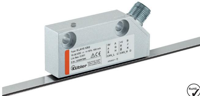
The non-contact absolute magnetic linear measurement system Limes LA10 / BA1 - made up of the sensor head LA10 and of the magnetic band BA1 - reaches a resolution up to 1 µm with a maximum distance of 0.2 mm between the sensor and the band (incl. masking tape).
